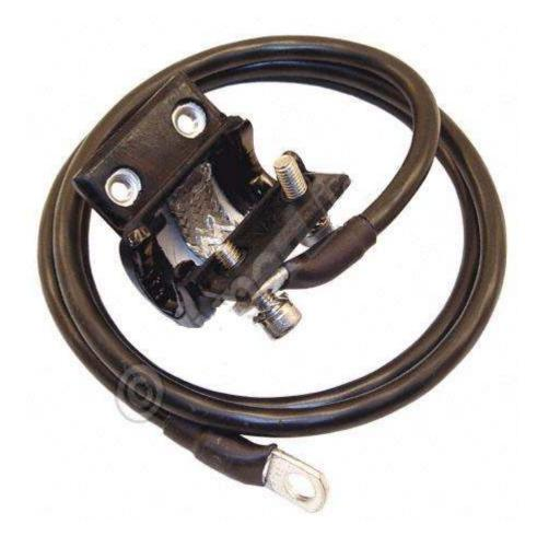
Grounding Kits are a cost effective way to provide grounding on 400 Series coax cable. These kits are fast and easy to install and feature a pre-formed grounding strap with integral butyl mastic which helps ensure a weatherproof splice. This is designed for use with 400-series coax cable from manufacturers such as CommScope® (WBC-400), Times Microwave Systems® (LMR-400) and Altelicon<sup>™</sup> (CA-400).
