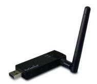
To protect your wireless connectivity, the high-speed wireless USB adapter can encrypt all wireless transmissions through 64/128-bit WEP data encryption and also supports WPA and WPA2(AES)
