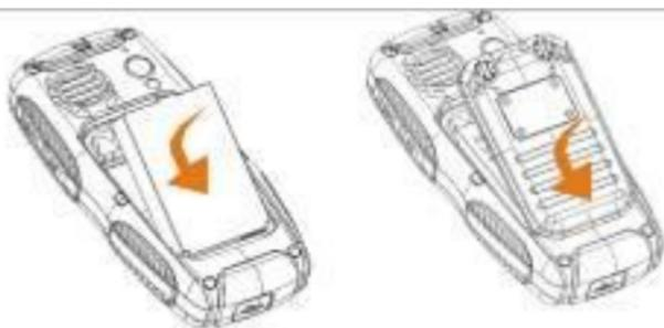
2. Inserting the battery cover to the slot, revolve the battery screw to horizontal direction.
