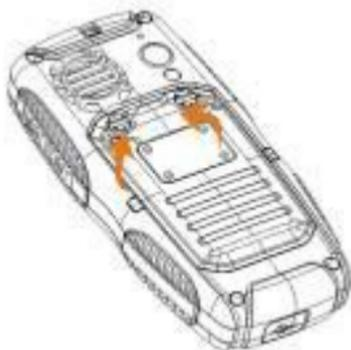
3. Confirm the battery well installed before power on.
